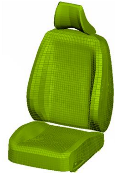
Chalmers generic LS-Dyna model of the test set-up used in the AHBM 2 and AHBM 3 tests with volunteers
